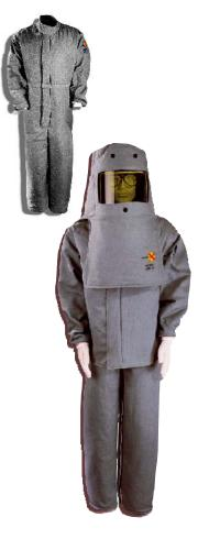
Oberon's ARC25 suit is designed to provide protection from arc flash heat exposures. The suit exceeds the requirements of NFPA 70E Hazard Risk Category 3 (HRC3), up to 29 cal/cm². Oberon's ARC25 suit is manufactured with 80% inherently FR aramid, and 20% melamine. These high technology lightweight (up to 40% lighter than FRT fabrics) and proprietary fabrics can reduce heat stress. All materials used in the construction of these garments are inherently flame resistant, including the thread.
